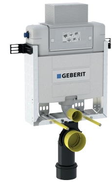
Geberit Alpha Kombifix, low height 12 cm, top / front operated 6/3L flush.
